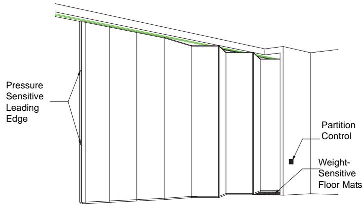
Note: The Hufgard system may be ordered with only the pressure sensitive leading edge, only the weight-sensitive floor mats, or a combination of both.
