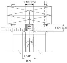
Type 50 clear anodized aluminum track. Shown exposed. Optional for Series 3100, 3500, & 3900 widths to 20'0" OR heights to 10'0" [6.09x3.04]. If either dimension is exceeded, use alternate track type. Not available for Series 4100.
