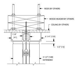
**Type 18 clear anodized aluminum track.** Includes built-in ceiling saver and header trim. Optional for all sizes. Must be exposed.
