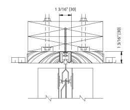
Type 50 clear anodized aluminum track. Shown recessed. Optional for Series 3100, 3500, & 3900 widths to 20'0" OR heights to 10'0" [6.09x3.04]. If size of either dimension is exceeded, use alternate track type. Not available for Series 4100.
